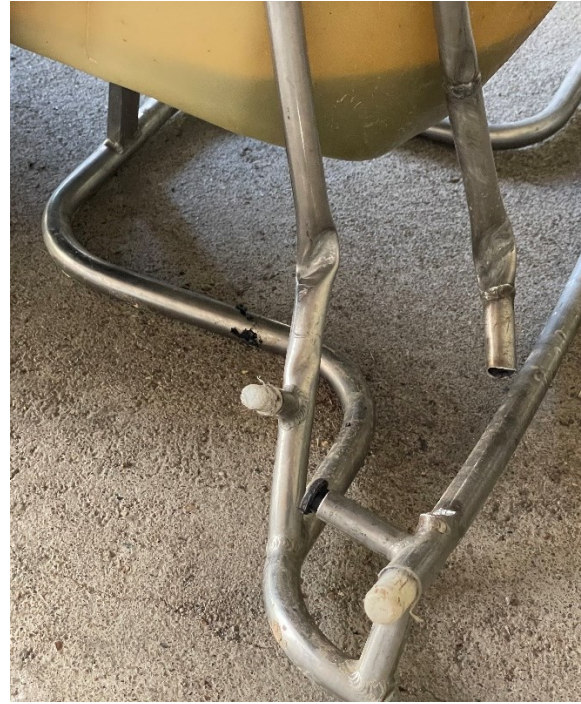
Figure 3: marks on paramotor chassis from contact with one of the power line cables (source: BEA)
