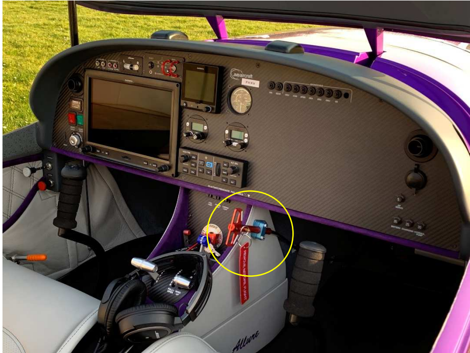
Figure 3: VL-3 cockpit with airframe parachute activation handle (source: BEA)
