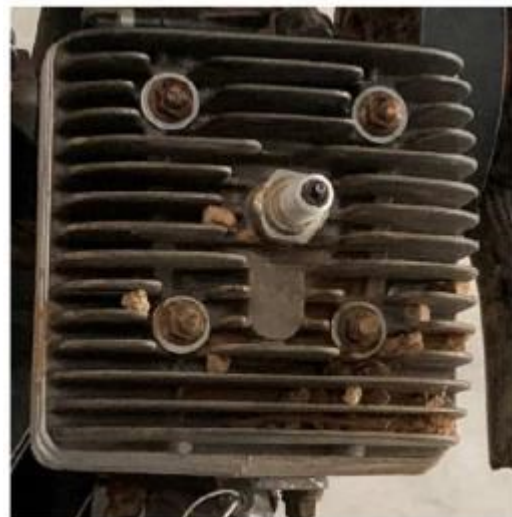
Figure 4: stones caught between the fins of the engine cylinder head (Source: BEA)
