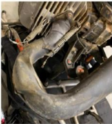
Figure 3: exhaust system distortion (Source: BEA)
