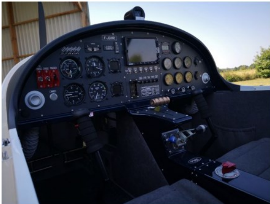
Figure 3: view of fuel selector in Viper SD4 cockpit in "left" position (source: Aquilair Aircraft)
