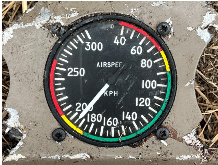
Figure 1: airspeed indicator blocked at 195 km/h (source: BEA)
