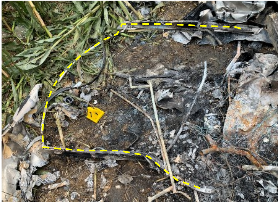
Figure 6: canopy frame (source: BEA)
