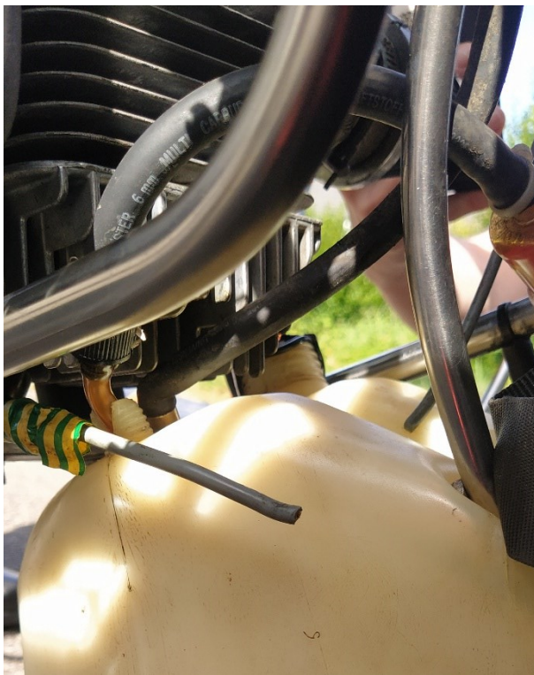
Figure 1: spark plug wrapped in insulating tape, cut power cable (Source: BEA)
