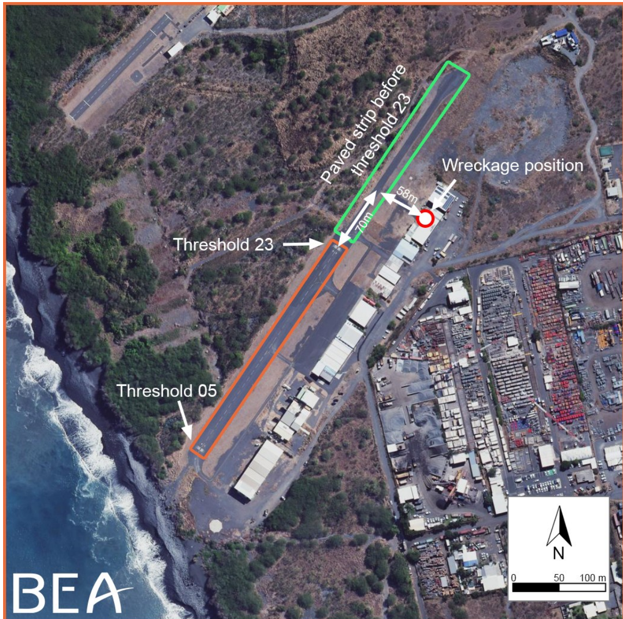
Figure 1: position of wreckage (source: Géoportail, annotations BEA)
