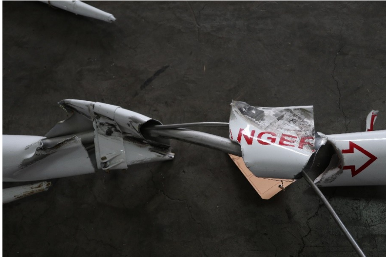
Figure 4: marks resulting from contact of the rotor blades with the tail boom (source: BEA)
