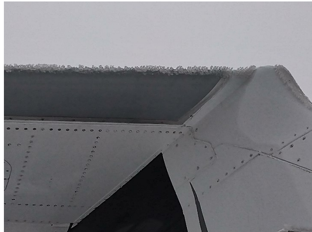
Figure 3: icing on the leading edge of the elevator still present 3 h after the accident (source: BEA)
