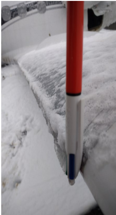
Figure 2: icing on the leading edge of the left wing still present 3 h after the accident. The white on the upper surface of the wing is the residue of the product used by the fire-fighters (source: BEA)
