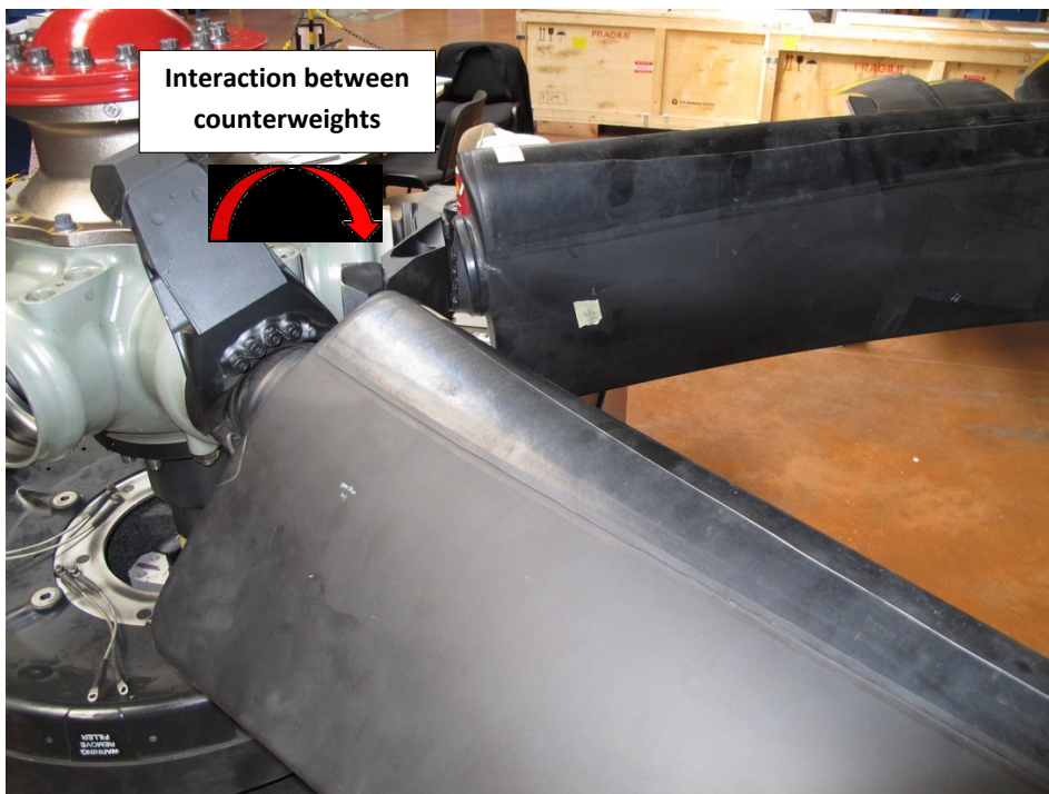
Figure 21: Interaction between the counterweight of blade 4 and the counterweight arm of blade 5
