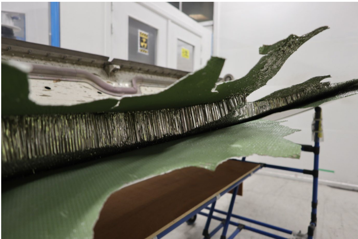
Figure 4: trailing edge of Slat No 2 of the A380 A6-EOM (source: BEA)
