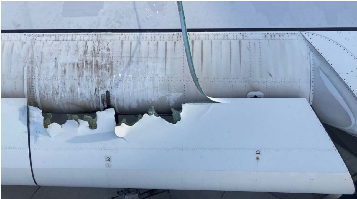
Figure 2: leading edge slat No 2 before disassembly (source: Airbus)
