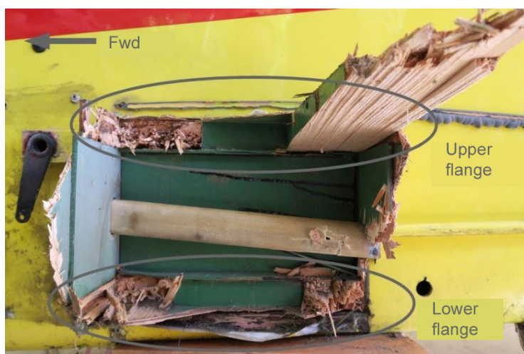
Figure 2: View of the area of the wing spar failure, photo taken facing the fuselage
