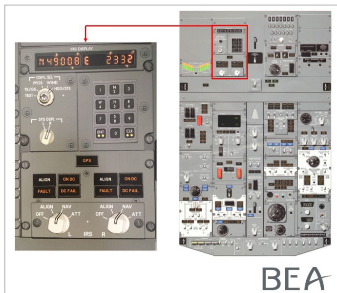
Figure 6: IRS FAULT light on IRS Mode Selector Unit on overhead panel
