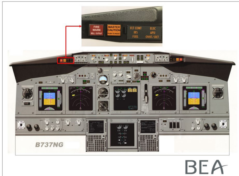
Figure 5: "Master Caution Push to Reset" light and annunciator with IRS light on left instrument panel
