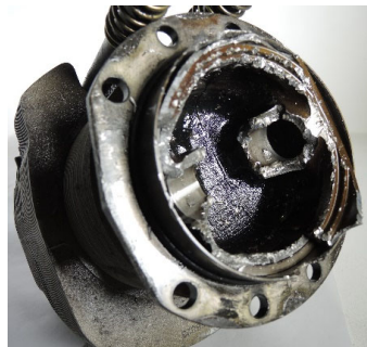
Figure 6: Partially destroyed piston blocked in cylinder
