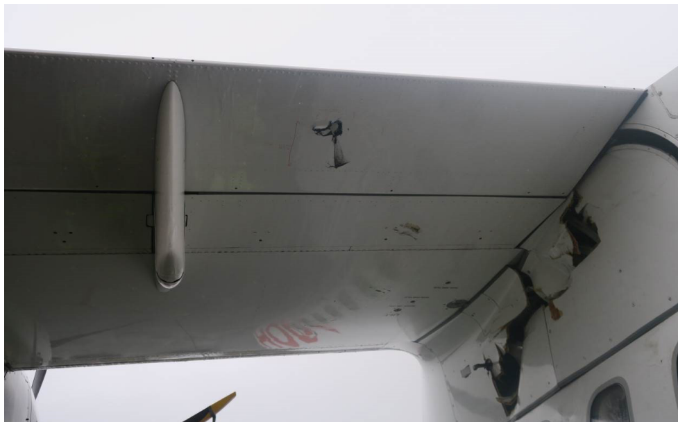
Figure 2: Damage to the flap
