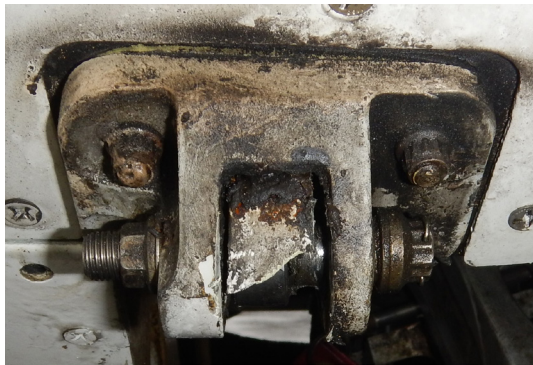
Figure 3: Remaining part of rear hinge assembly
