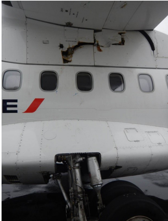
Figure 1: Wing fairing damage and missing L MLG door
