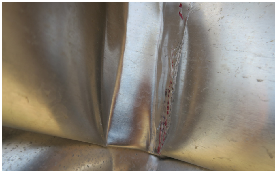
Figure 3: Detail of depression of the leading edge of the right wing of 57YM and traces of red paint
