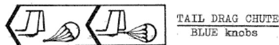
Figure 6: presentation of the pictograms associated with the drag chute control lever in the flight manual
