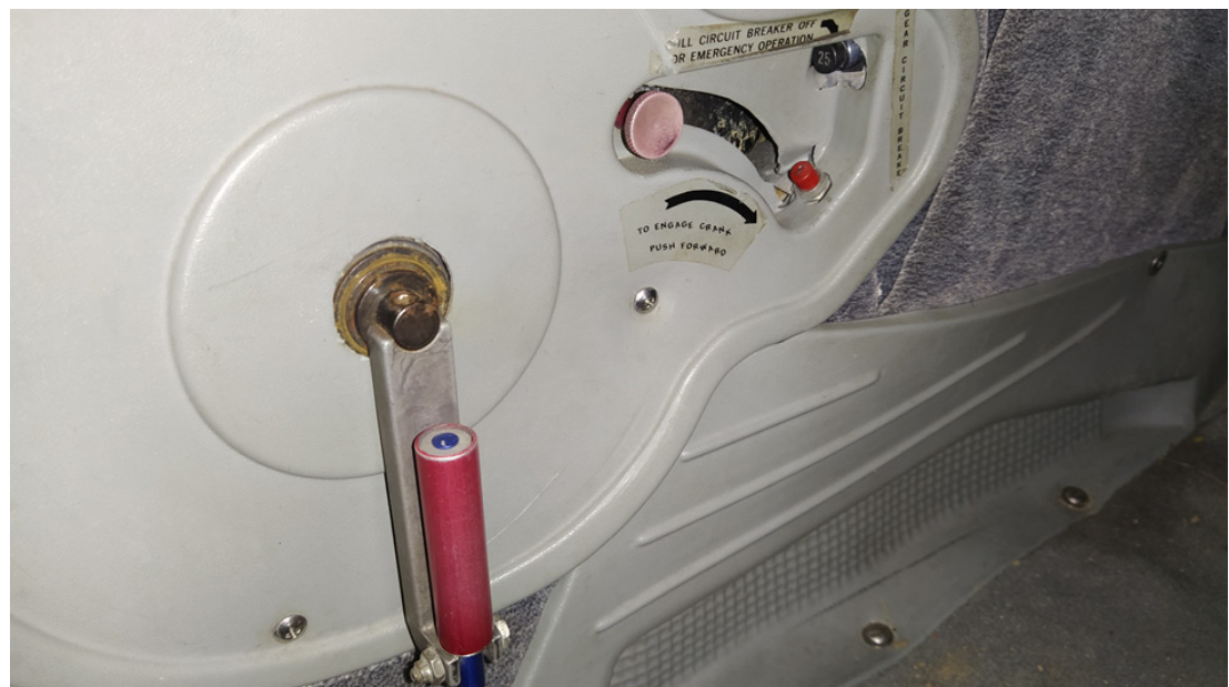
Figure 1: emergency landing gear extension handcrank (view from bottom of pilot's seat)
