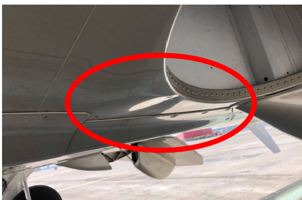
Figure 6: Deformations observed on lower surface of left wing
