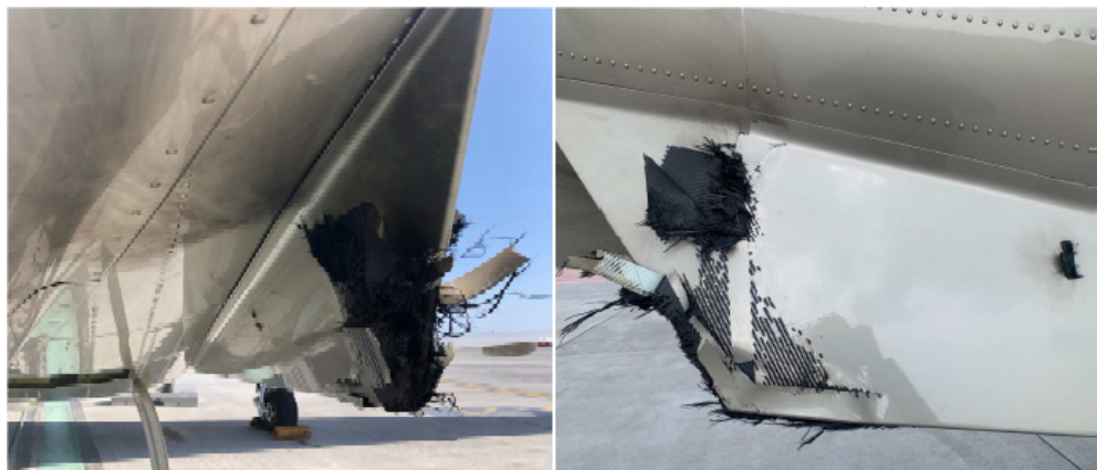
Figure 3: Damage observed on right ventral fin
