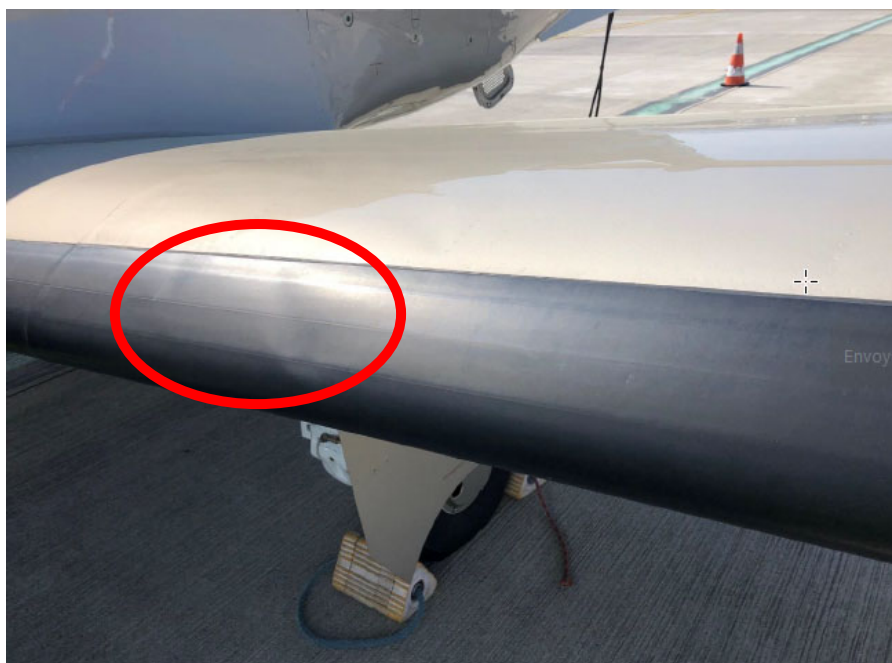
Figure 5: Deformations observed on left wing leading edge
