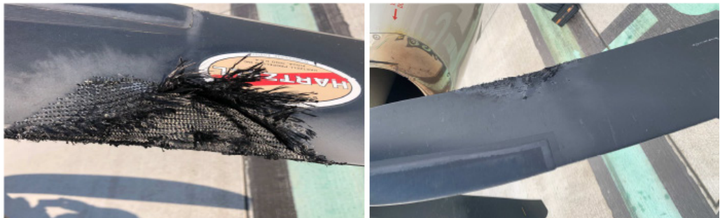
Figure 2: Damage observed on a propeller blade
