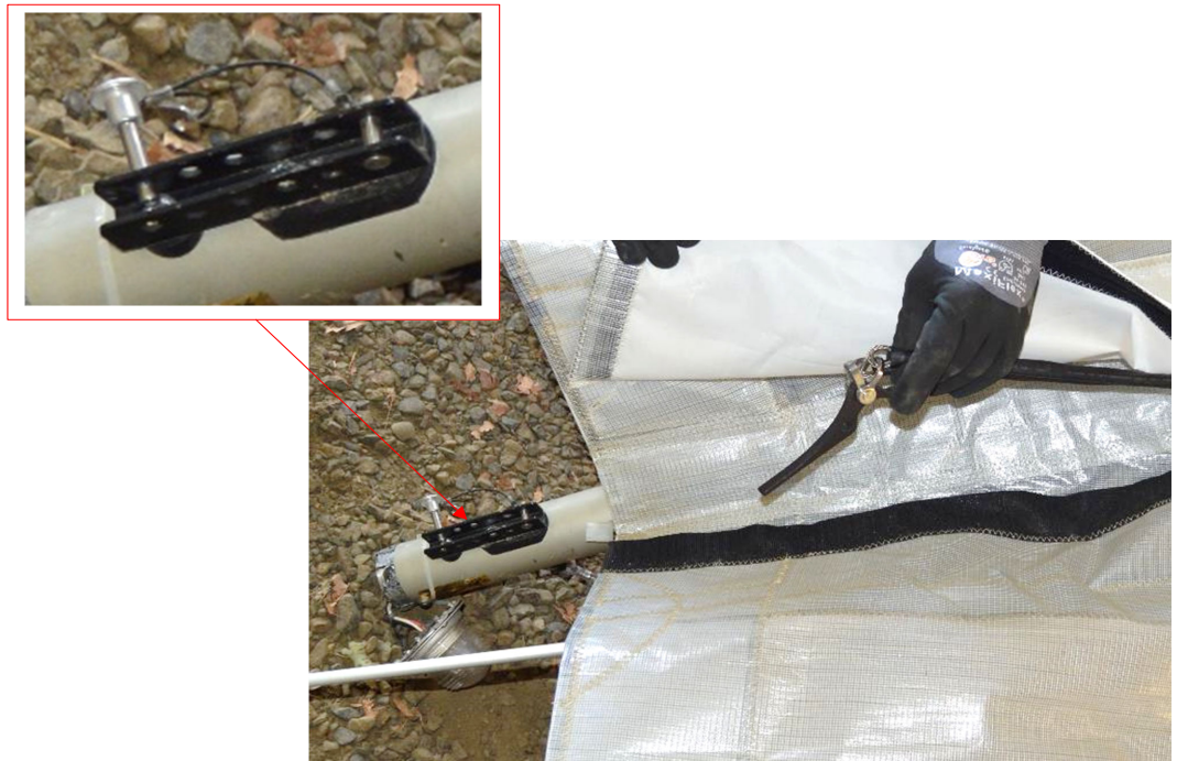
Figure 4: Tautening system as it was found on the wing
