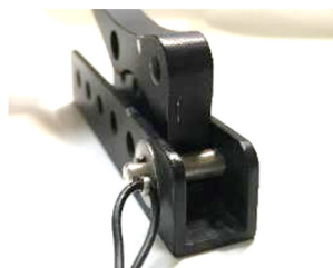
Tip slipped under fixed pin
