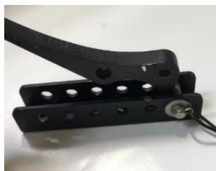
Hook tip slipped under fixed pin of hanger
