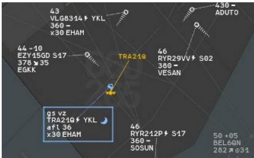
Figure 6: illustration of track marker (in amber) and of F-PASD (in blue) displayed during the serious incident to PH-YHC (source: DSNA)
