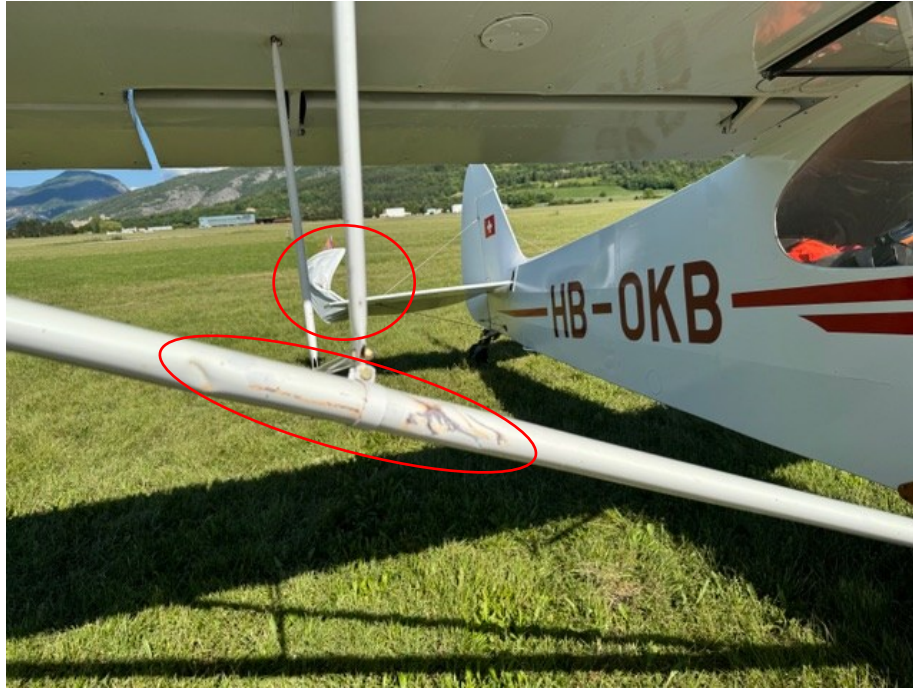
Figure 2: damage observed on aeroplane (source: instructor, annotations BEA)
