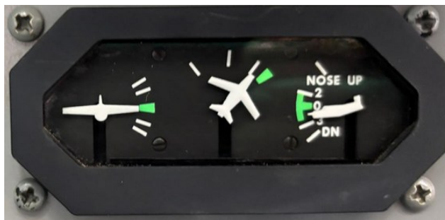
Figure 6: recreation of display in cockpit of trim positions at time of collision with ground (source: BEA)
