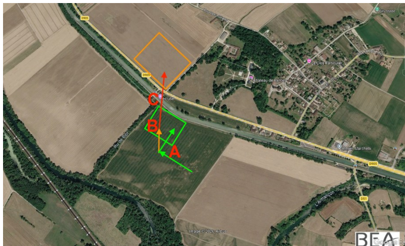
Figure 3: initial field (in green) then final field (in orange) chosen by the pilot. The green arrows indicate the initially planned base leg and final approach.
