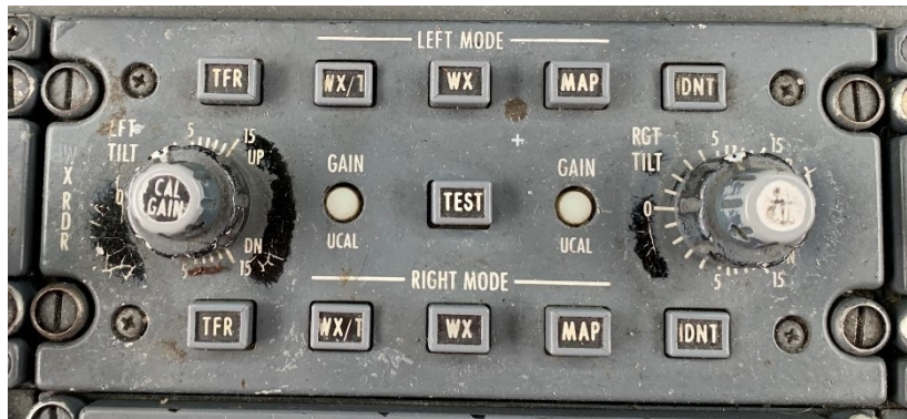
Figure 6: EC-NLS radar control panel photographed after the accident (Source: BEA)
