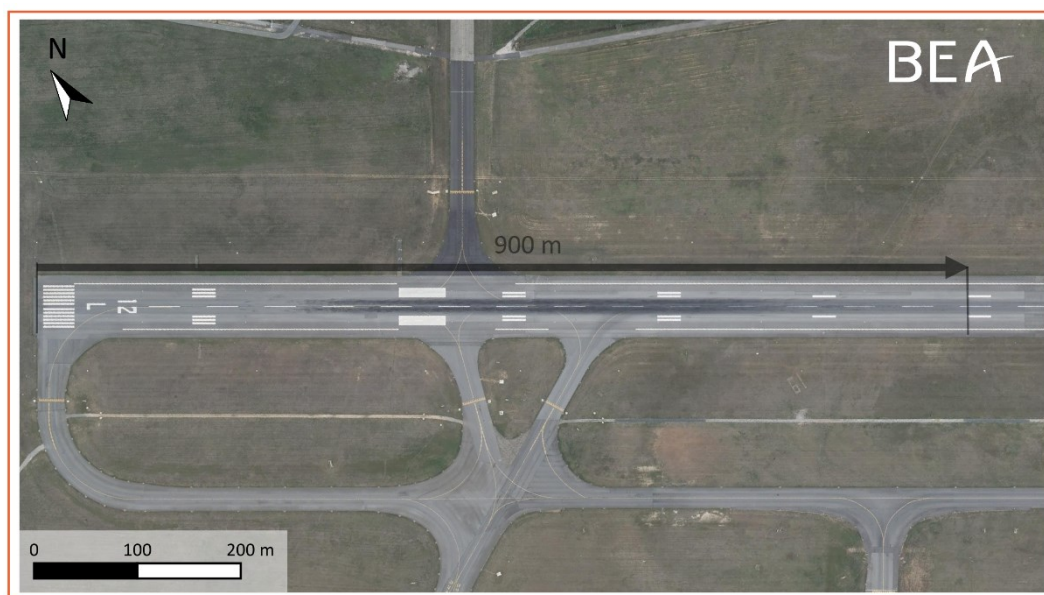
Figure 14: runway 12L, TDZ marking
