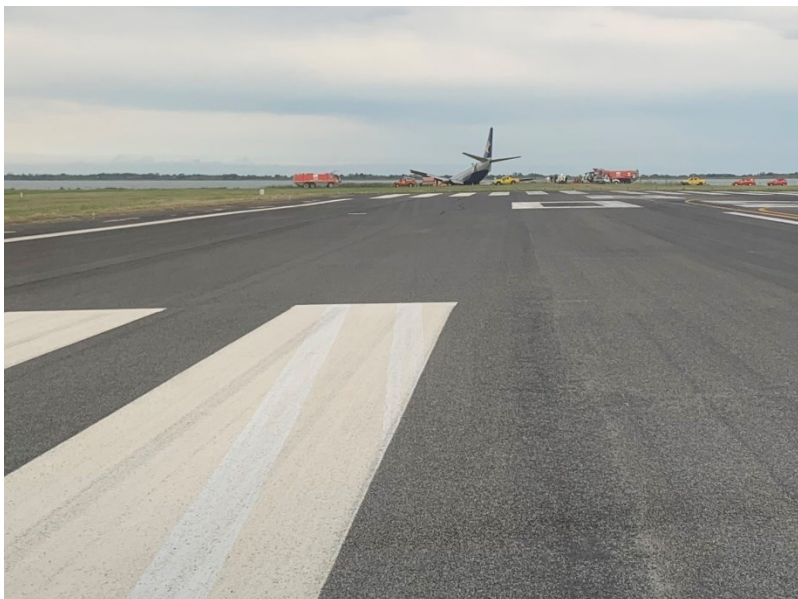
Figure 18: marks similar to a case of vapor cleaning (Source: BEA)
