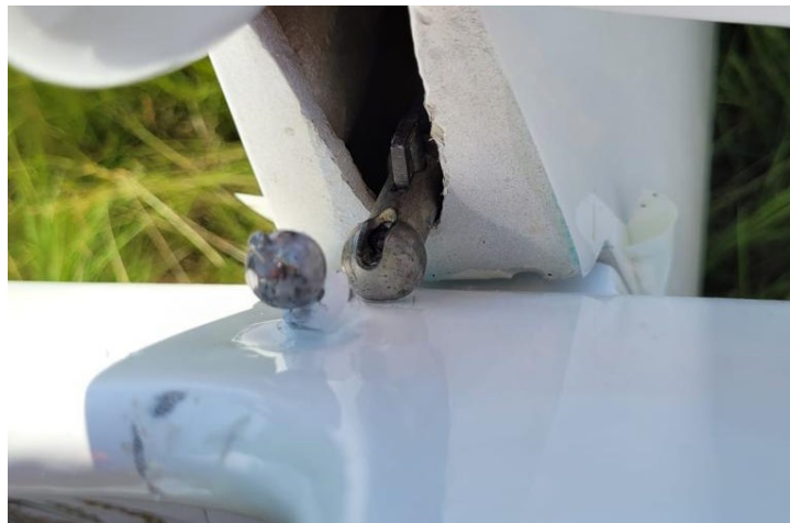
Figure 2: ball and socket connector found disconnected (source: GTA)
