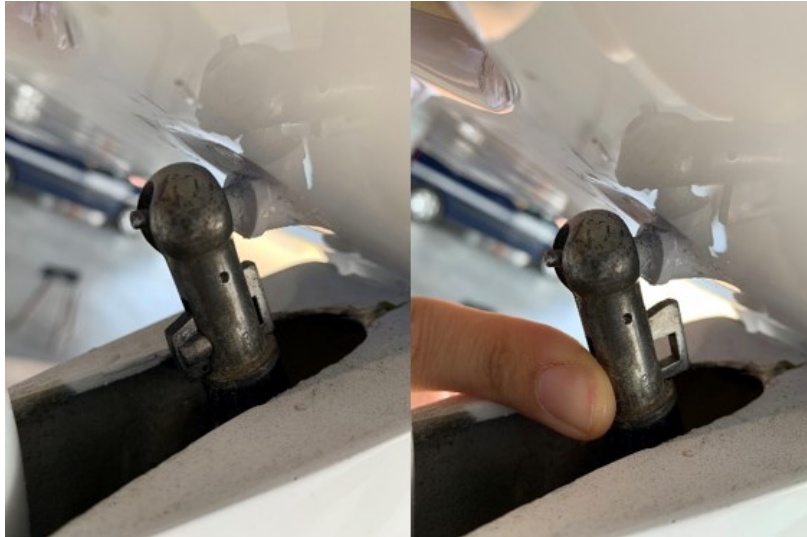
Figure 4: locked and unlocked positions of ball and socket connector (source: BEA)
