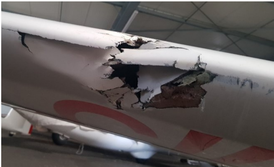
Figure 2: damage on the leading edge of the left wing
