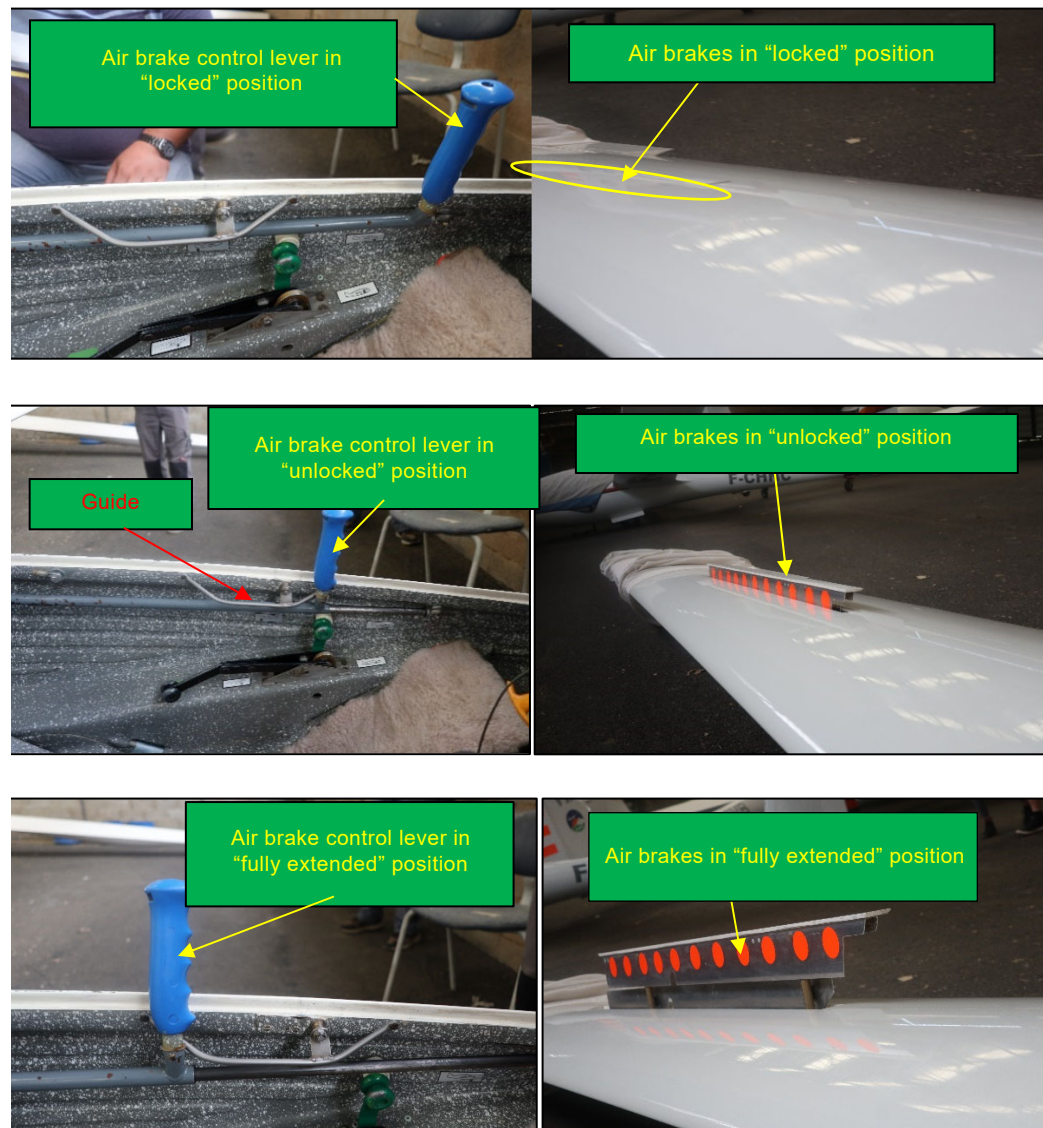
Figure 3: air brake control positions
