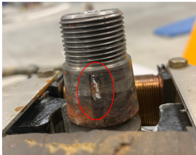
Figure 3: sheared keyway at end of crankshaft (source: BEA)
