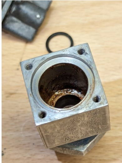
Figure 4: opened right-hand bleed valve (source: BEA)
