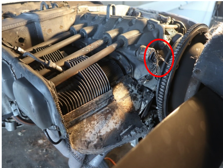
Figure 2: oil pressure sensor (Source: BEA)
