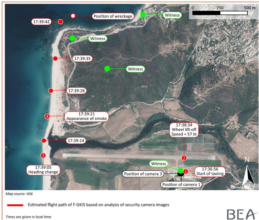
Figure 1: reconstruction of aeroplane's path
