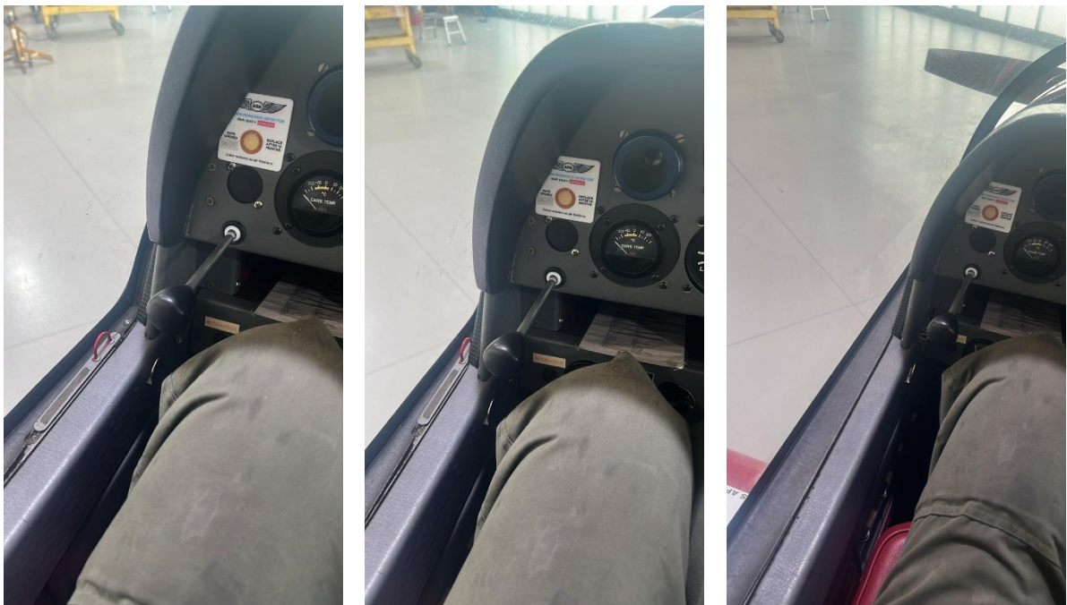
Figure 3: photo of release lever from left seat with canopy closed (left-hand side), open by 8 cm (middle) and open by 30 cm (right-hand side) (source: BEA)
