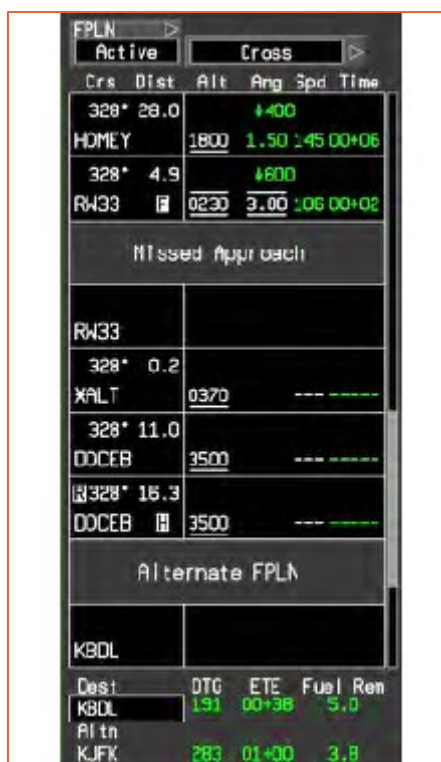
Figure 13 : WAYPOINT LIST (Source : Dassault Aviation)
