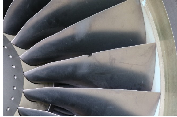
Figure 11: example of damage observed on engines (source: BEA)
