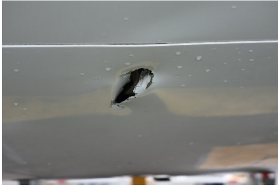
Figure 10: example of damage observed on the airframe (source: BEA)
