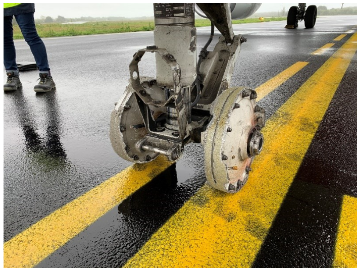
Figure 9: ruptured wheels of nose landing gear (source: BEA)
