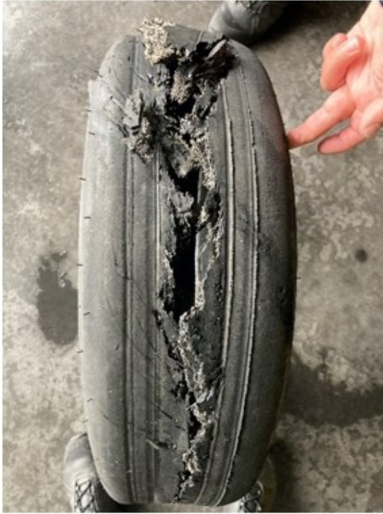
Figure 7: burst tyre (source: BEA)
