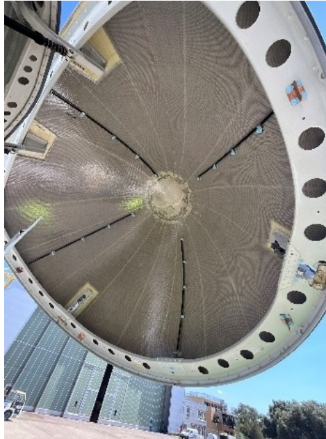
Figure 3: damage on inner face of radome (source: Air France)
