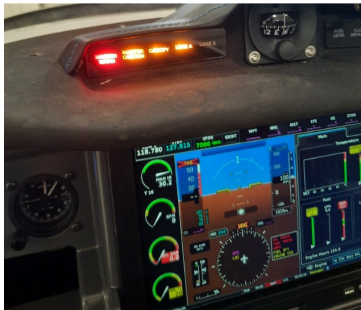
Figure 8: warning and caution panel on F-HCDN (source: BEA)
