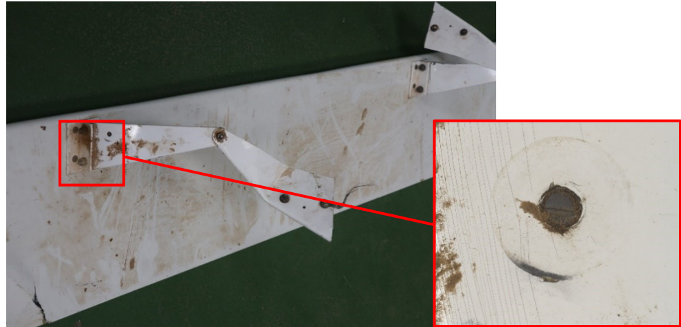
Figure 4: left flap arm and end of rod attaching screw in position in bore hole (source: BEA)
