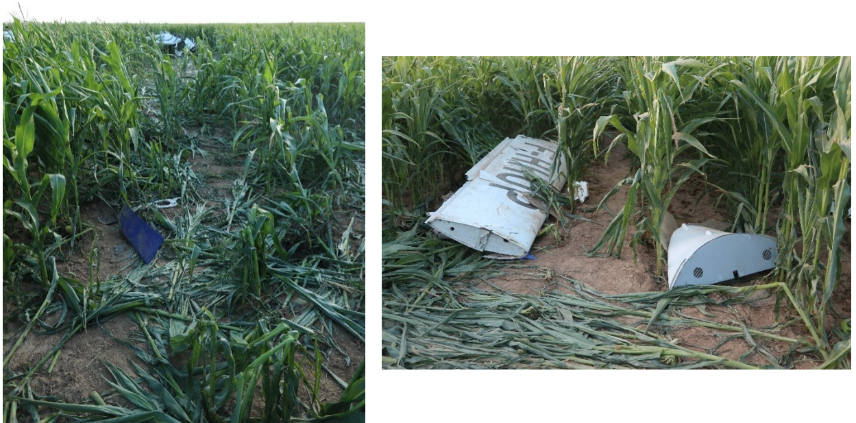
Figure 3: views of wreckage from initial impact point (on left), and left wing found between the first point of impact and the main wreckage (on right) (source: BEA)
