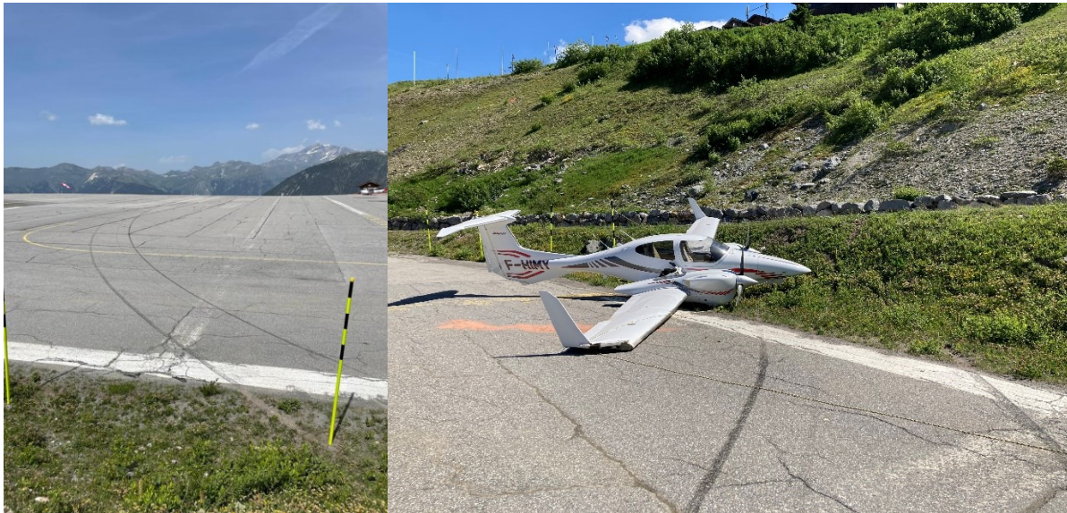
Figure 3: photo of braking marks (on left) and of aeroplane (on right) (source: BEA)
