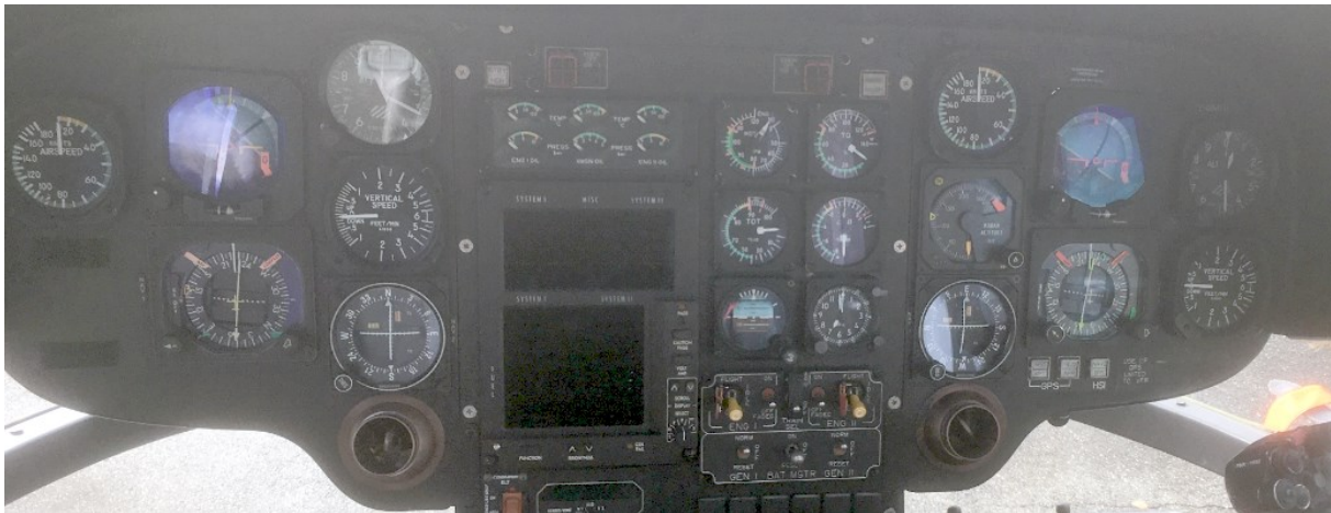
Figure 3: instrument panel of an EC135-T1 similar to F-HJAF (source: BEA)
