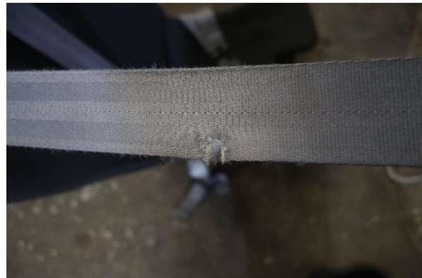
Figure 15: mark on harness right strap of front left seat (source: BEA)
