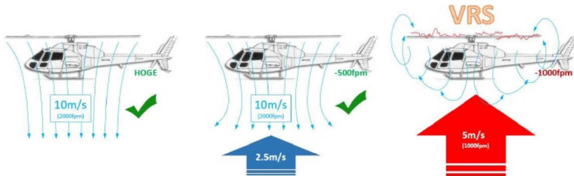
Figure 3: description of the conditions in which a vortex ring state occurs (Source: Airbus, SIN No. 3123-S-00)
