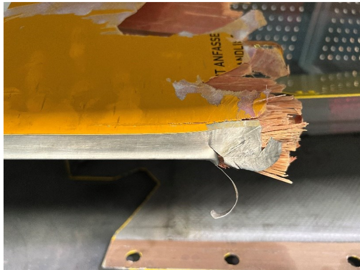
Figure 5: damaged leading edge (source: BEA)
