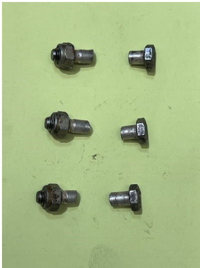
Figure 6: ruptured bolts (source: BEA)
