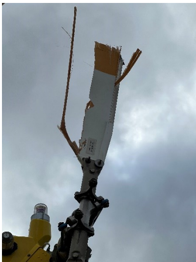
Figure 4: delaminated blade (source: BEA)
