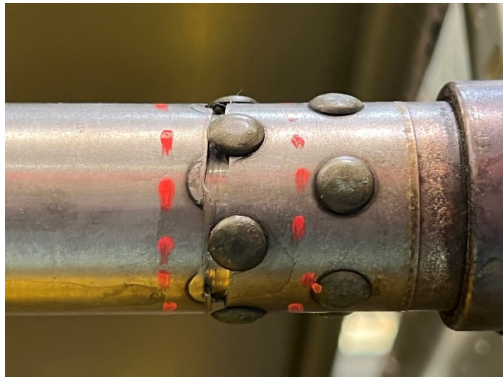
Figure 7: ruptured rivets (source: BEA)
