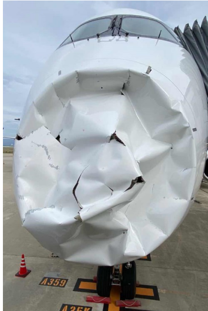
Figure 4: damage to the radome (Source: Air France)
