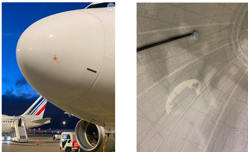
Figure 37: bird strike and debonding of the inner skin of an A318 radome (Source: Air France)
