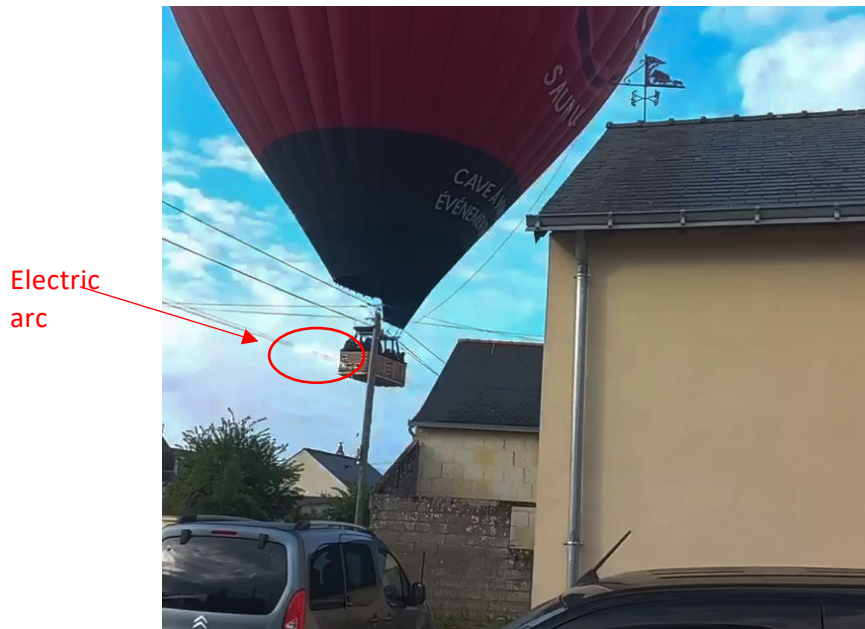
Figure 2: excerpt from video at time of collision (Source: witness on ground, annotated by the BEA)
