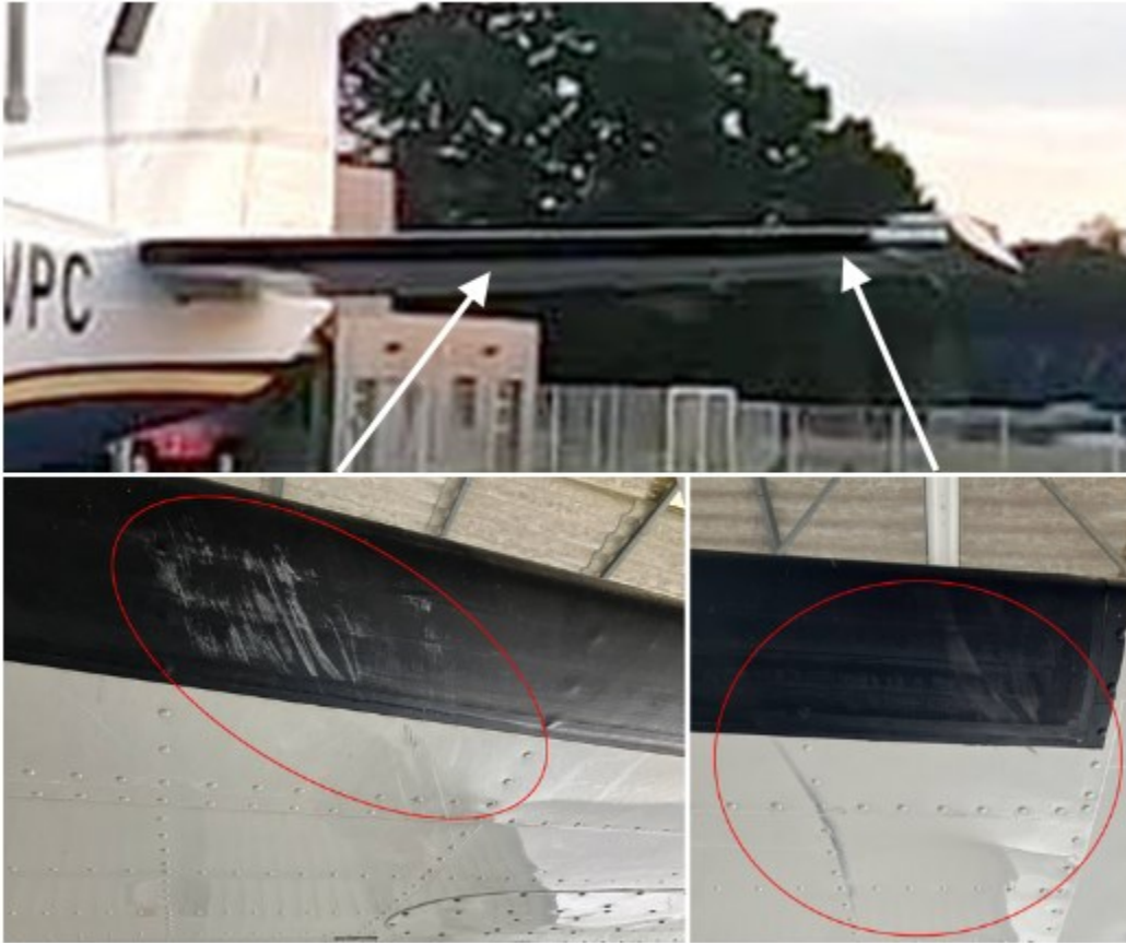
Figure 2: marks on leading edge and lower surface of left-hand horizontal stabilizer. (source: BEA)
