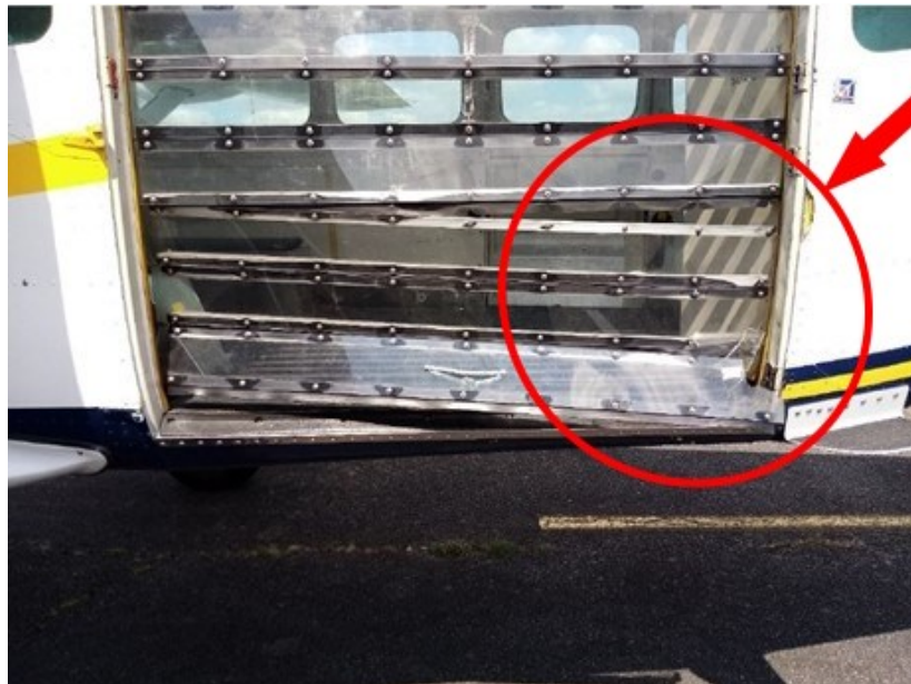
Figure 1: damage to door (jamb and slats) (source: skydiving school)
