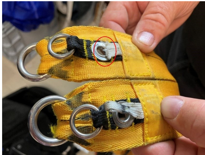
Figure 3: view of the left (bottom) and right (top) risers with the broken textile loop (source: BEA)
