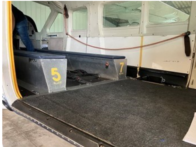
Figure 7: layout inside the airframe in skydiving activity configuration (source: BEA)
