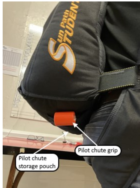
Figure 5: position of pilot chute storage pouch on a parachute of the same type (source: BEA)
