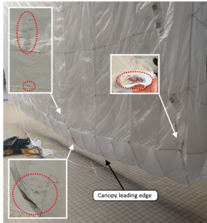
Figure 4: damage to leading edge and right-hand tip of reserve canopy (source: BEA)
