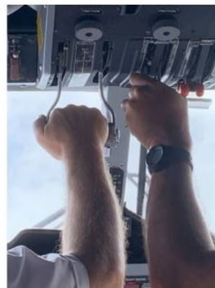
On the approach, the PF manages the power, the PM selects the propeller speed
