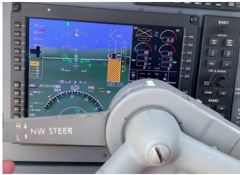
Figure 10: photo of NWS lever aligned although the gear is not locked in the centred position (source: BEA)
