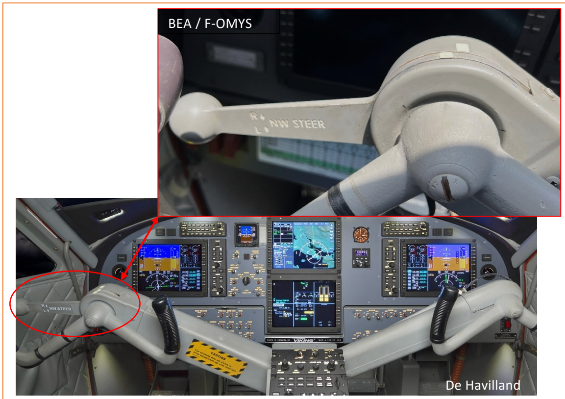
Figure 3: NWS lever (source: De Havilland / BEA) 7
