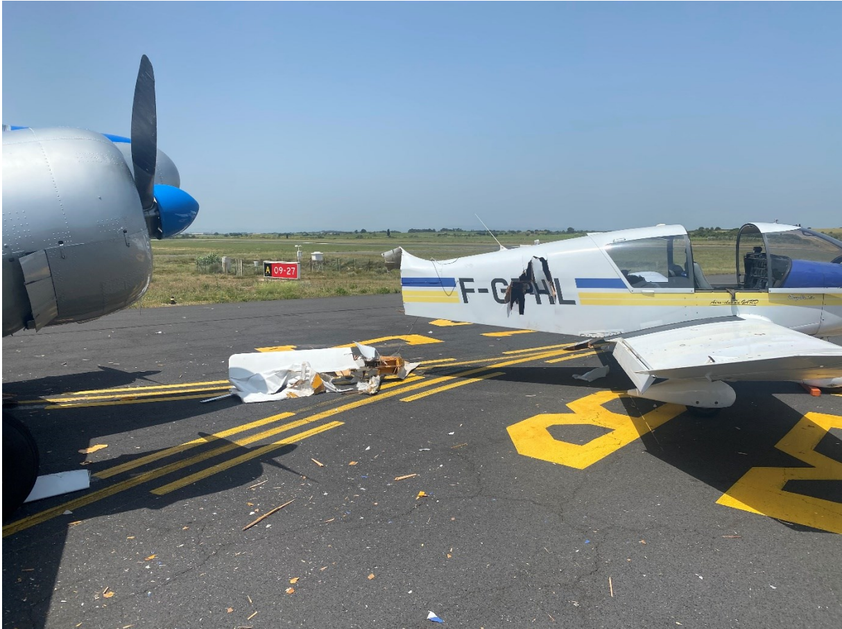
Figure 2: damage to F-GPHL (source: pilot of HB-GAC)
