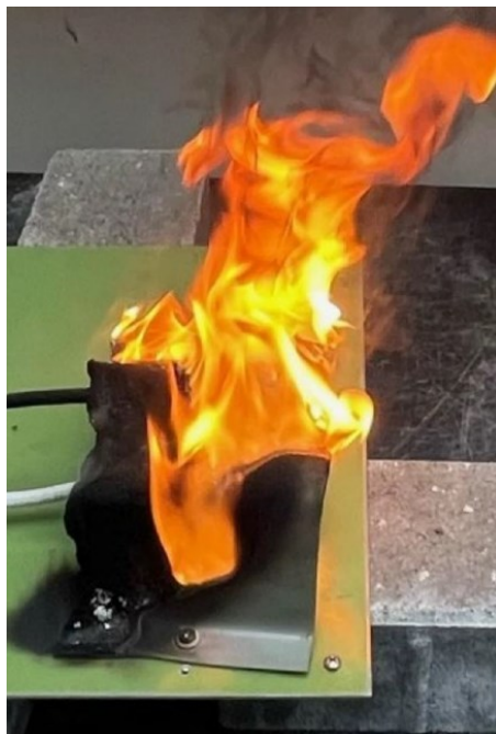
Figure 19 : capot en ABS se consumant (Source : CONCORDE BATTERY CORPORATION)
